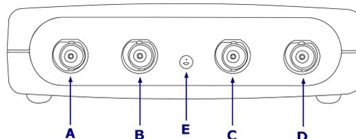
**A. Ch A.** Input channel A. Similarly for channels B, C and D.
